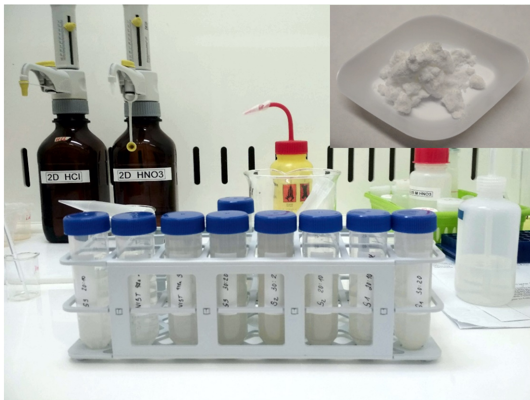
Figure 7. The final stage of precipitation. The ascorbic acid is added, and the samples are prepared for centrifugation. The ascorbic acid powder prepared for dissolution in DIW and further used for precipitation of Ag is displayed in the upper right corner.
