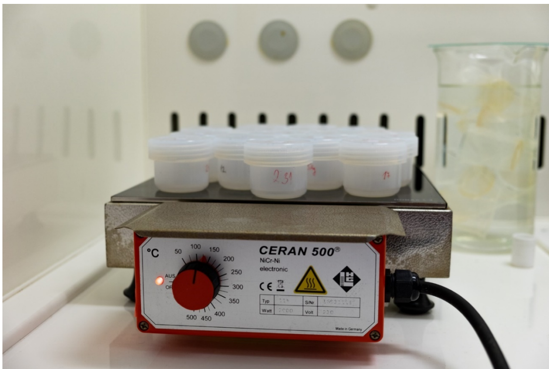
Figure 6. Samples dissolved on a hot plate in closed Savilex beakers at 120–130 °C for 24–48 hours.
