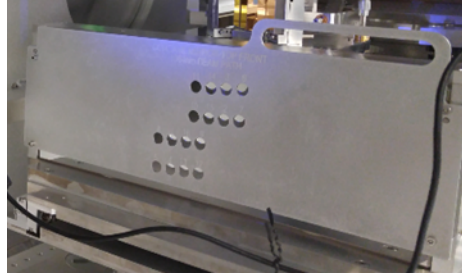
Figure 6.16: Aluminum alignment plate placed in front of the concave mirror. Each hole represents one reflection off the mirror.
