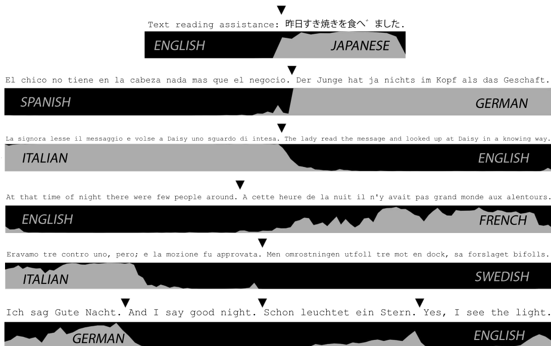
Figure 2.3: Illustration of text partitioning. The black triangles indicate true boundaries of languages. The black part shows probability of detecting the language labeled in gray color, and the gray part shows complement for the second language since in this setup we restricted our model to use only the two languages in question. The misclassification of Italian and German as English in the last two examples may reflect increased noise in our English training data.
