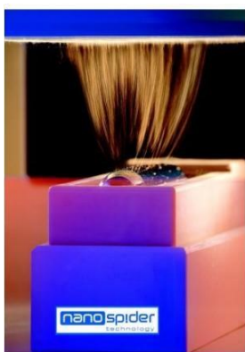
Figure 7.1 A thin layer of polymer solution film (b) is raised by a metal roller (a), which is at the same time the positive electrode. This electrode is partially submerged in the polymer solution (c), and nanofibers are created between the spinning electrode and the collector (f, negative electrode) due an extremely high-intensity electrostatic field (e). The solvent evaporates and the fibres stretch at room- or elevated-temperature and are collected by a polypropylene non-woven fabric (d) on the negative electrode (f). Sources: NY Times 2012 (left image), Kubinová et al. 2009 (right image)
