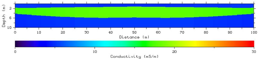
Figure 2: Inversion result from 9-configurations synthetic EM data from Example 4.
