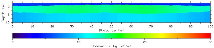
Figure 3: Inversion result from 9-configurations synthetic EM data from Example 3 with 5% white noise added.
