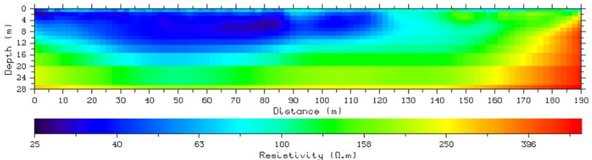
Figure 5: Inversion result from ERT data measured in a crop field over a contact between alluvial sediments and outcropping crystalline basement, near Bystrice.
