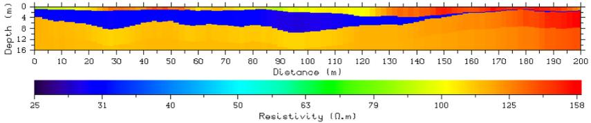
Figure 4: Inversion result from 6-configurations EM data measured in a crop field over a contact between alluvial sediments and outcropping crystalline basement, near Bystrice.
