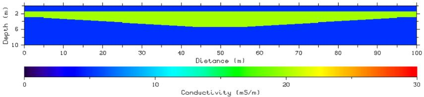
Figure 1: Original model of a 3-layered earth with a resistive middle layer and descending bottom layer.
