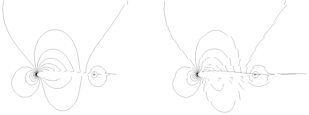
Figure 8.5: Isolines of the Mach number for mesh M1 and third polynomial order (left), and M3 and first polynomial order (right) - inviscid flow M = 0.5 , \alpha = 2^\circ
