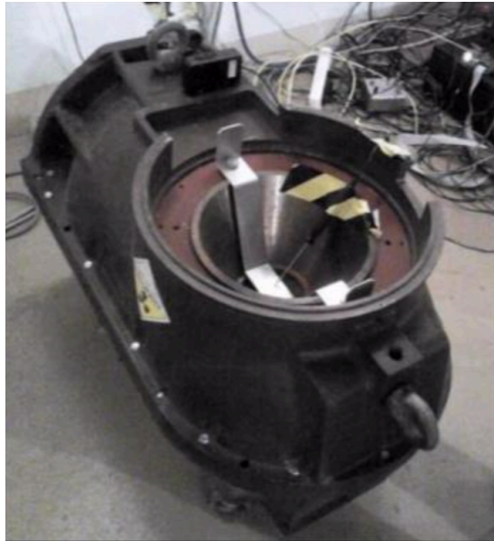
Figure 5.4: Terabalt Cobalt-60 source at UJP Prague [31].
