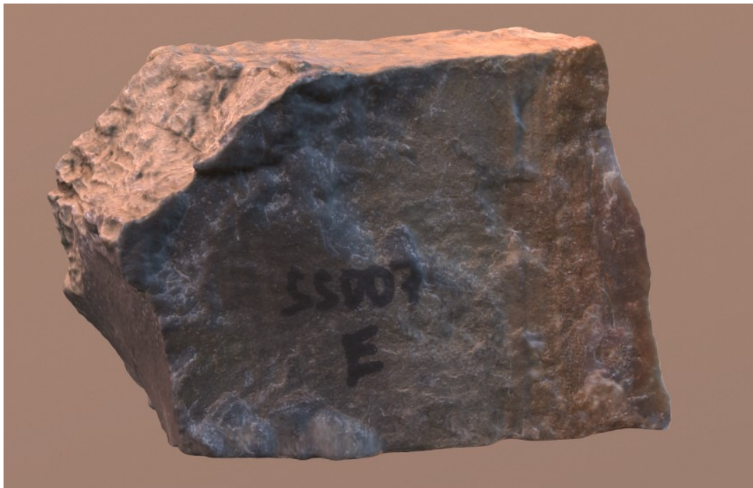
Figure 5. 3D model of sample “SS007E” done by Author of the thesis using Agisoft Photoscan software.
