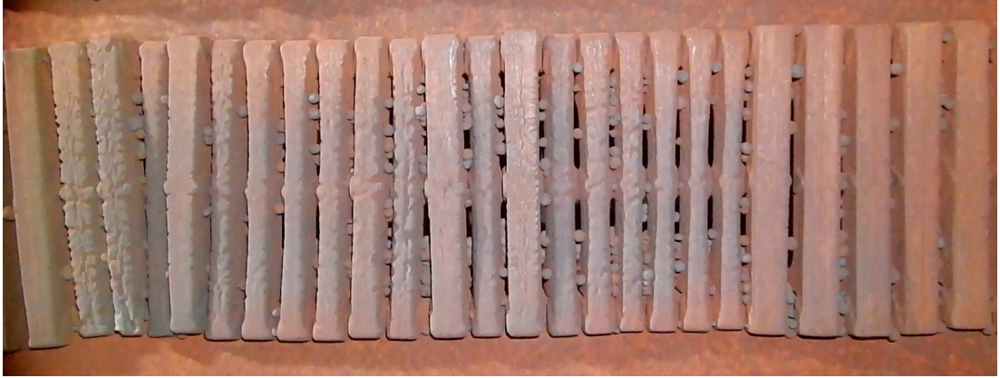
Figure 4.1: Pellet car with rounded (degraded) ribs.
