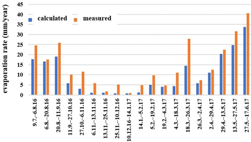
Fig. 4. Example of comparison between calculated and measured values of evaporation rate.
