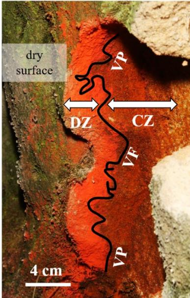
Fig. 3. Visualization of the vaporization plane depth by uranine powder coloring method. DZ – diffusion zone (dark orange), CZ – capillary zone (red), VP – vaporization plane (the transition between DZ and CZ). Modified from Weiss et al. (2018).
