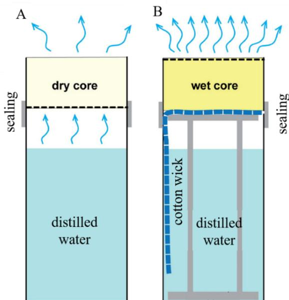
Fig. 2. Evaporation apparatuses for measuring evaporation rate: a) dry core with the vaporization plane at the bottom base of the core, b) wet core with the vaporization plane at the upper base of the core. The vaporization plane position is visualized by the dashed line. Modified from Bruthans et al. (2018).
