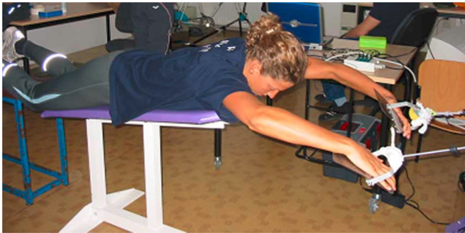
Figure 4. Initial position on the isokinetic swim bench for the exhausting 30-s test using the butterfly arm stroke (Ganter et al., 2007)
