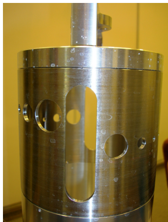
FIG. 11: The photo of the beam reducer with different apertures to define the diameter of the diagnostic beam
