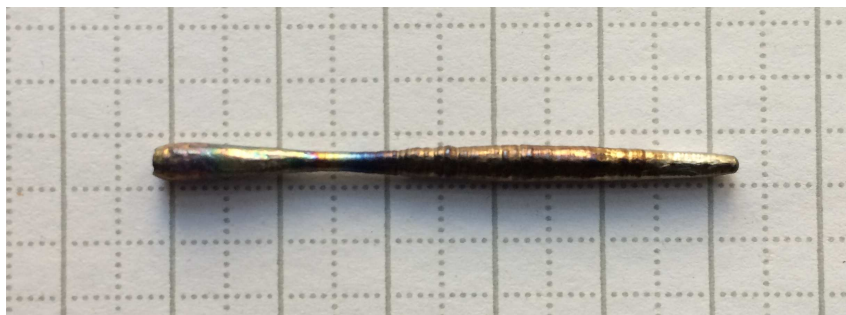
Figure 3.1: The JM018 ingot of \text{CeCo}_{0.715}\text{Si}_{2.285} grown by Czochralski process in a triarc furnace. The dotted lines on the underlying surface are in 5mm distance.
