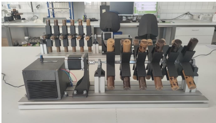
Figure 10. Laboratory-constructed rotating devices for the tightly bound soil water extraction (Institute of Hydrodynamics, CAS).
