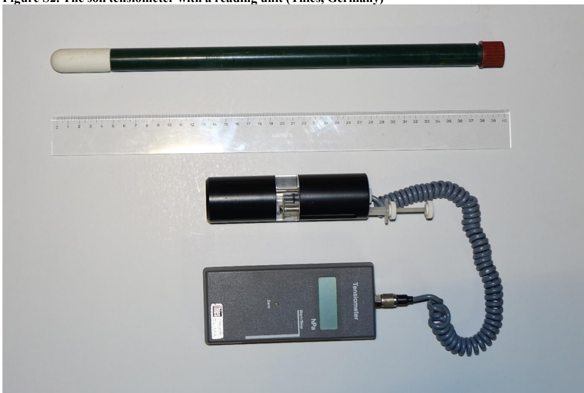
Figure S2. The soil tensiometer with a reading unit (Thies, Germany)
