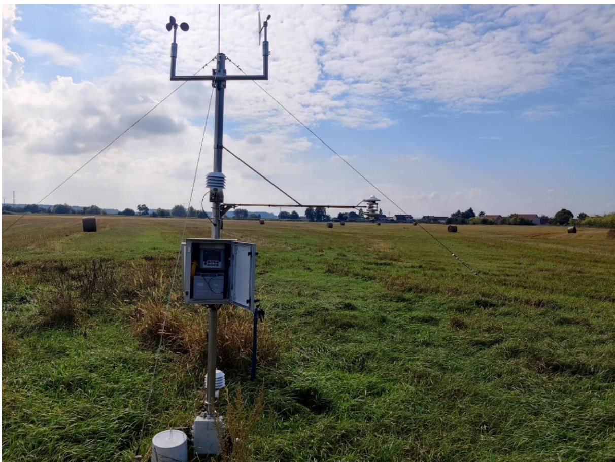
Figure 8. Monitoring station at the experimental site Zvěříněk used for soil moisture and meteorological data collection.
