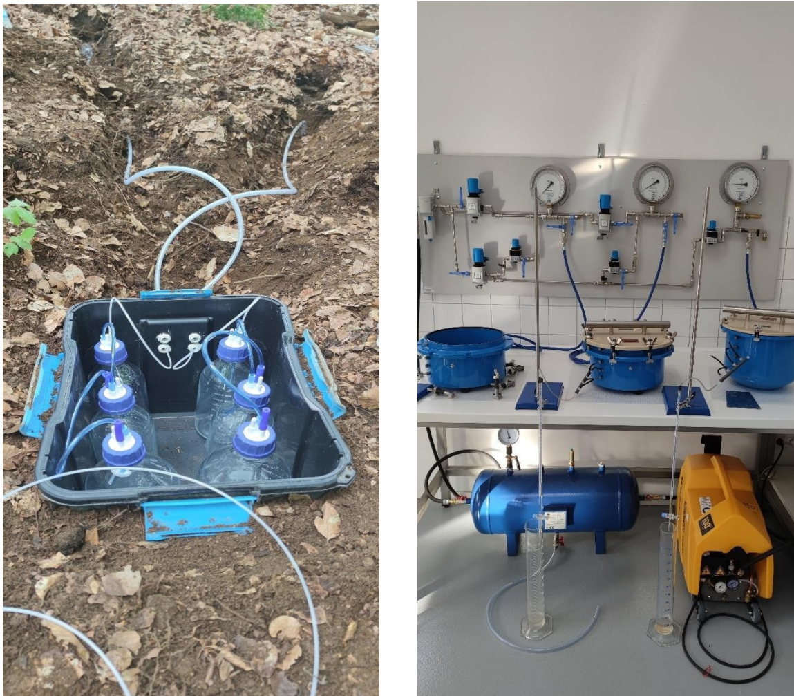
Figure 9. On the left: the installed VS-Pro system for sampling mobile soil water at the Bohemian Forest National Park site. On the right: pressure plate apparatus for extracting the mobile soil water fraction from soil samples (Institute of Hydrodynamics, CAS).
