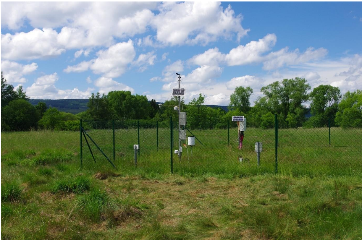
Figure 7. Monitoring station at the experimental site Trhové Dušníky used for soil moisture and meteorological data collection.
