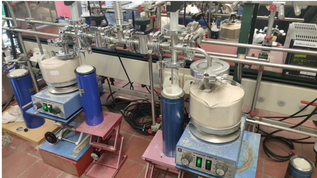
Figure 2. The CVE apparatus at Forschungszentrum Jülich, Germany, used to extract water from soil samples. The sample is heated in a sand bath, and the resulting water vapour is condensed in blue thermos flasks cooled with liquid nitrogen.
