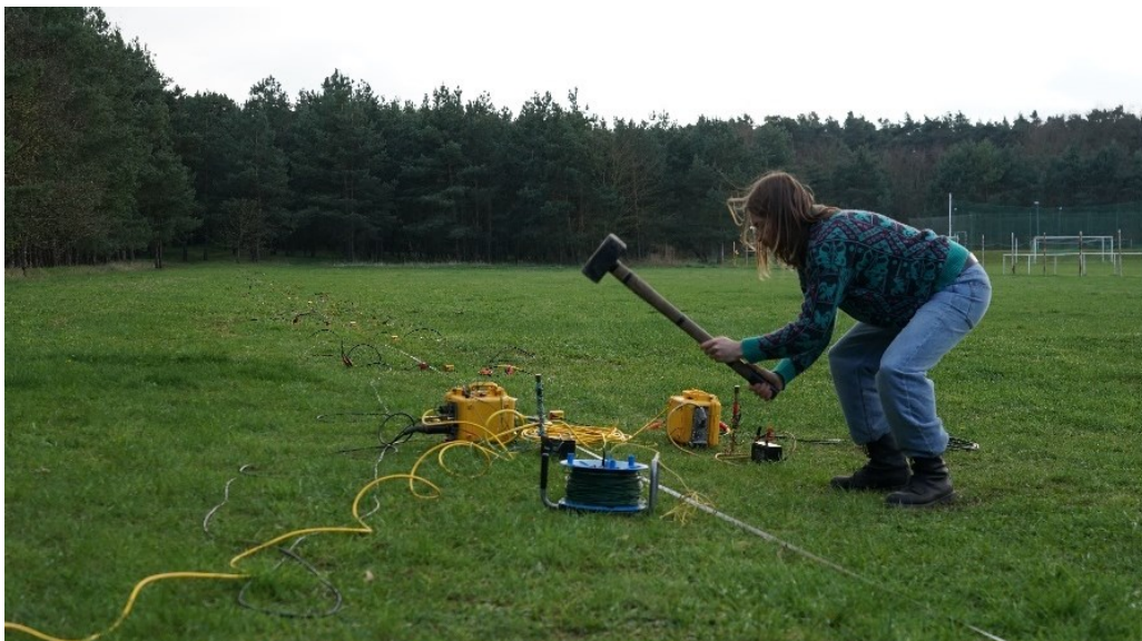
Figure 49: Field photo of active MASW data acquisition using simultaneous recording with horizontal and vertical geophones and a sledgehammer as the seismic source.
