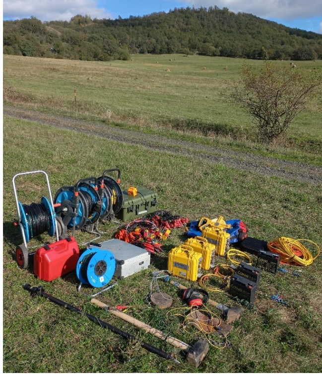
Figure 34: Illustrative setup of a Geometrics seismic array, including horizontal, vertical, and 3C geophones, seismic cables, Geodes, sledgehammers, steel plates, trigger cables, a notebook, GNSS receiver, and additional accessories. This configuration can be used for seismic refraction, reflection, and most types of surface wave analysis.
