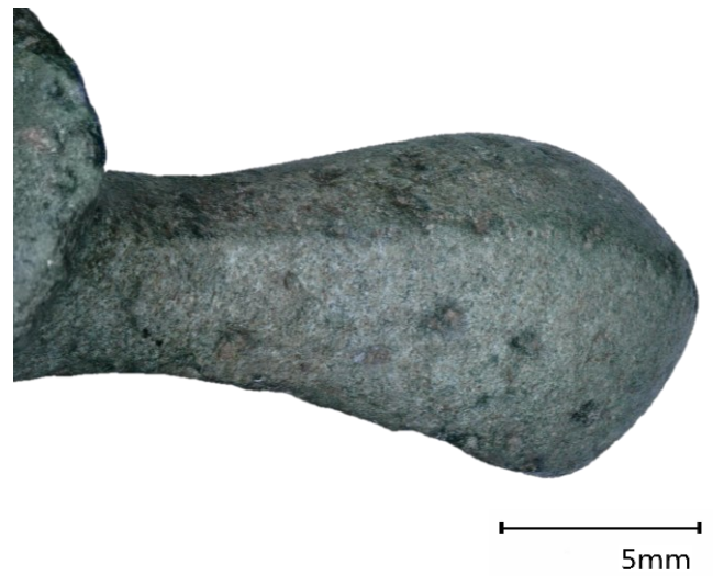
Fig. 28.: Casting flash on the body of cat. no. 58, captured by Keyence VH 5000
