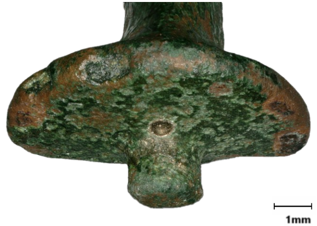
Fig. 43.: Retained casting knob, cat. no. 42, captured by Keyence VHX 5000
