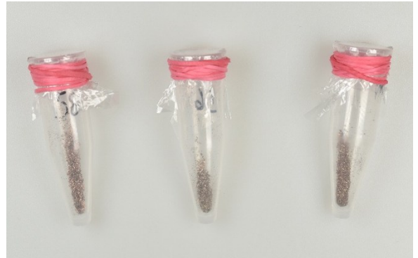
Fig. 22. Samples in Eppendorf test-tubes prepared for XRF analysis
