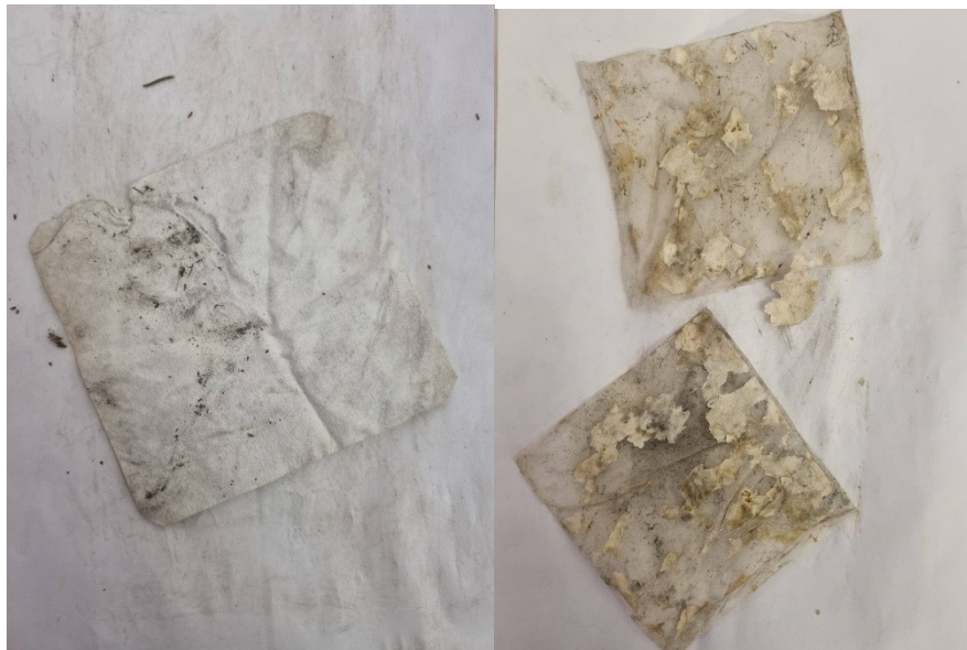
Figure 12: Reduced filter paper removed from the LS and HS plots, respectively in spring 2024. Filter paper is firmly attached to the nylon material from the HS plot.
