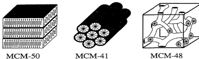
Figure 16: Schematic diagram of the structure of M41S family materials, MCM-50 (layered), MCM-41 (hexagonal) and MCM-48 (cubic). 26
