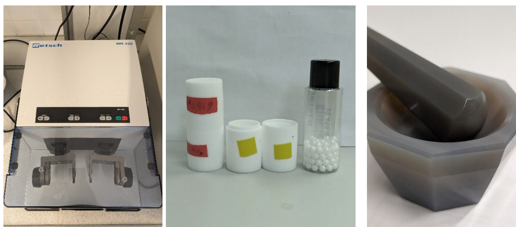
Figure 11. Images of the ball mill Retsch MM 400 Mixer Mill alongside PTFE grinding jars of volume of 10 ml and \text{ZrO}_2 grinding balls of diameter of 5 mm. The right image shows the mortar and the pestle.
