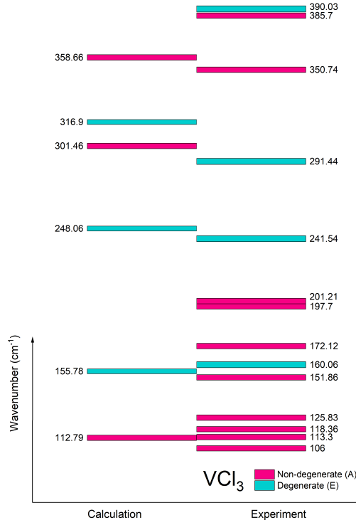
Figure 4.5: The comparison of calculated phonon modes and measured IR peaks for the R-3 structure at room temperature.
