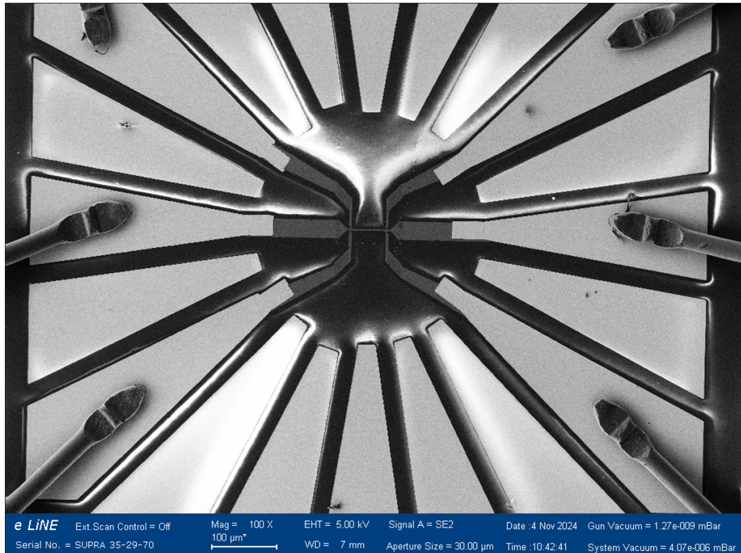
Figure 3.4 Scanning electron microscopy (SEM) image of the \text{Mn}_3\text{GaN} device (21-270_#1_A). Image taken by Zbyněk Šobáň.
