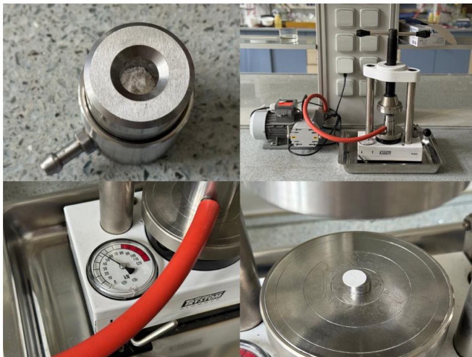
Fig. 15. Step-by-step preparation of pellets using hydraulic press
