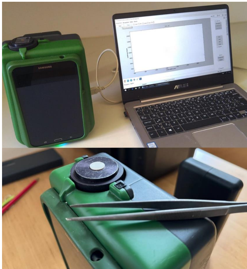
Fig. 16. EnSpectr RaPort handheld Raman spectrometer and process of measuring pellets
