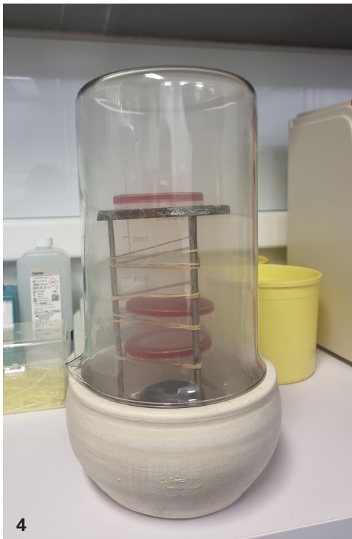
Fig. 4 Experimental setting for fumigating the testing plates and cultures in the Private Hospital Laboratory. The placement of the Petri plates before the initiation of the smoking process (fumigation under a 5000 ml beaker) is clearly visible.
