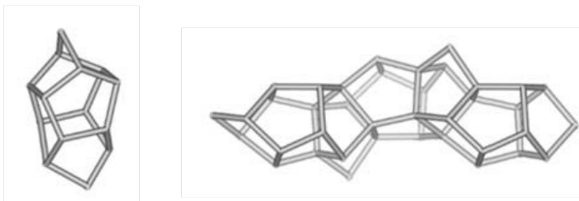
Figure 3: Building units of MFI framework type – pentasil unit (left) and pentasil chain (right). 1
