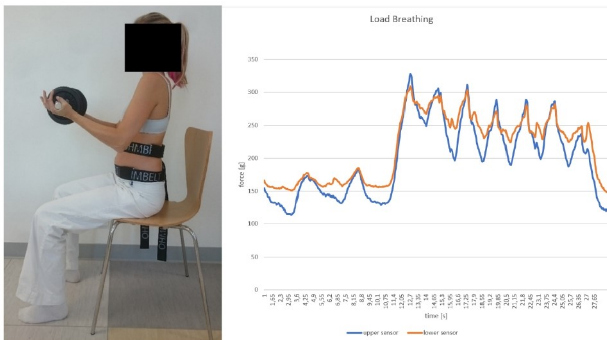
Fig. 3. Load breathing assessment. At the 10th second the weight was put into participant’s hands (note the steep increase of both lines in the graph).
