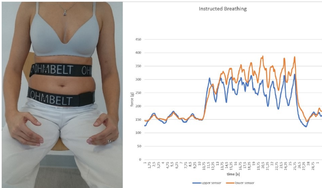
Fig. 4. Instructed breathing assessment. First, the individual breathes normally, then at the 10th second he/she was instructed to direct the breath towards both sensors (steep increase of both lines in the graph).
