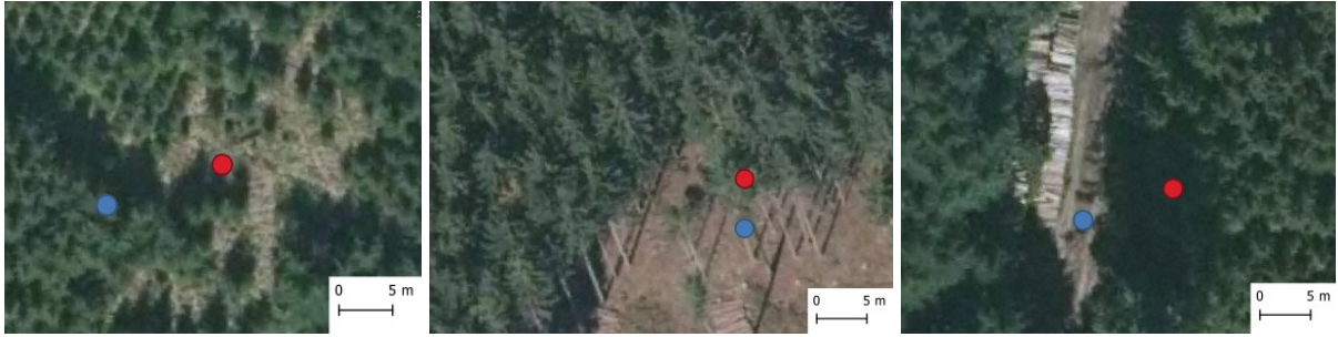
Fig. 10: The spatial comparison of L1B (blue) and L2A (red) footprint centroids from the same track.
