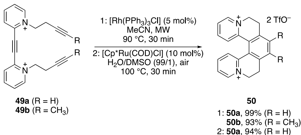
Scheme 16. First synthesized [5]helquats 50 using [2+2+2] cyclotrimerization.
