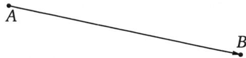
Figure 2.16: Global orientation of mesh edges based on a unique enumeration of vertices (here \text{index}(A) < \text{index}(B) ).
