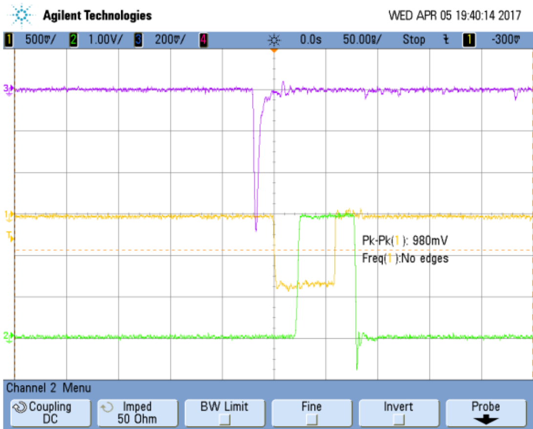
Figure 4.7: Negative analog signal from scintillator(purple), Negative digital signal from CFD(yellow), final Positive digital signal from TTL(green) [28]
