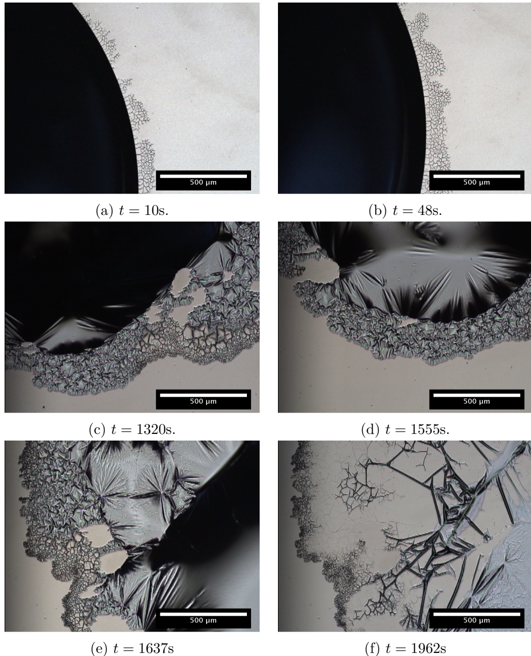
Figure 2.3: Evaporation of a penetrating water droplet with initial volume 3\mu\text{l} on a PTFE/Si surface at 30^\circ\text{C} . As the droplet permeates the surface, first branching arms formed and spread. Then, at a later time, the droplet lost its spherical shape as it permeated even further, forming rippling undulations. These further spread, and as the droplet evaporates, retracted. The state of the surface left behind by the droplet can be seen in Fig. 2.4.
