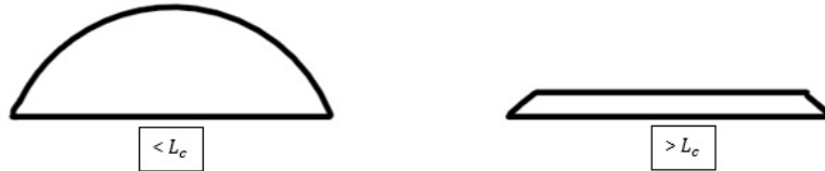
Figure 1.1: Microdroplet (left) with the length and height lesser than \lambda_c and a macrodroplet (right) with length higher than and height equal to \lambda_c (the two are not to scale). Taken from [24] with permission.
