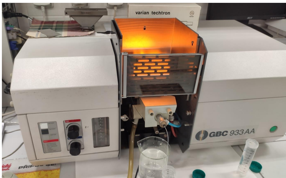
Figure. 2.1. A photograph of GBC 933 AA atomic absorption spectrometer.
