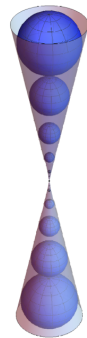
Figure 2.12: A cone of revolution as the envelope of one parameter system of spheres.
