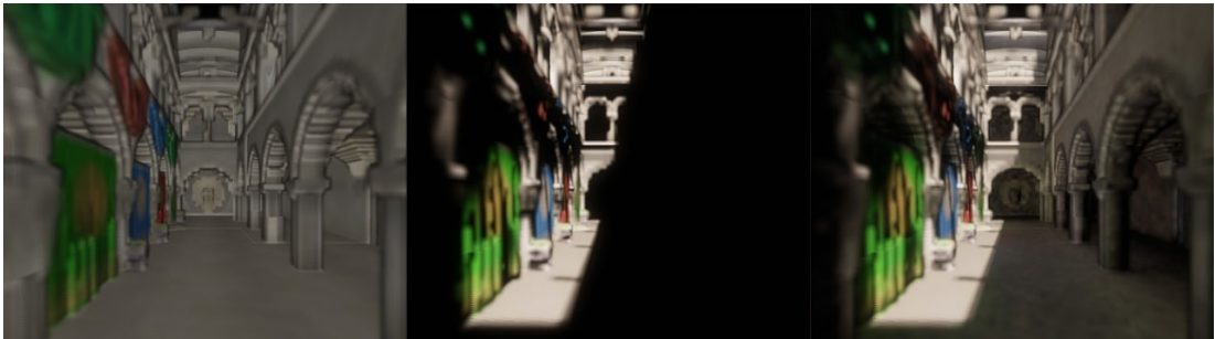
Figure 2.3: Albedo colours, direct light injection and light propagation. (Uyurkulak [2021])
