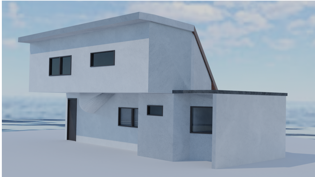
Figure 2.3: Planar faces get unnecessarily complicated if we use nurbs for modelling them. Some parts would needlessly suffer from poor quality if meshes were used for them, the overhand part 'holder' is modelled as a NURBS sphere combined with a conoid (ruled surface).
