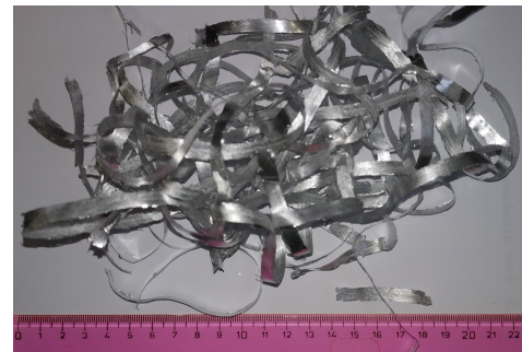
Fig. 1.9: An example of an alloy prepared by melt-spinning.
